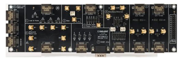
Figure 1 Ethernet Electrical Compliance Test Fixture Board
